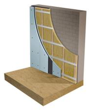
Mass air resonant frequency = 24Hz Panel size = 2.7m x 4.0m Partition surface area mass = 250kg/m2
